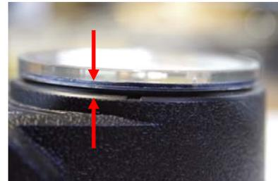
Now attach the new glass with adhesive. (for example: Loctite 401 or silicone adhesive Dreibond)
