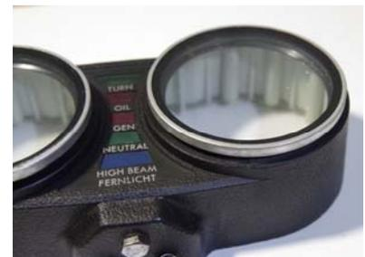
Clean up the [outer edges](#) of the raised lip with a file or sandpaper until you are able to push the new glass onto the protrusion.
